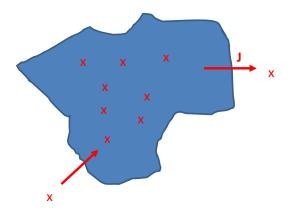
Consider the total charge Q in a volume V. This charge may vary as a function of time as charge is moving in and out through the boundary of the volume.
