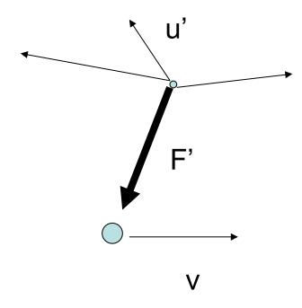
Source charge in motion produces velocity-dependent force on test charge
