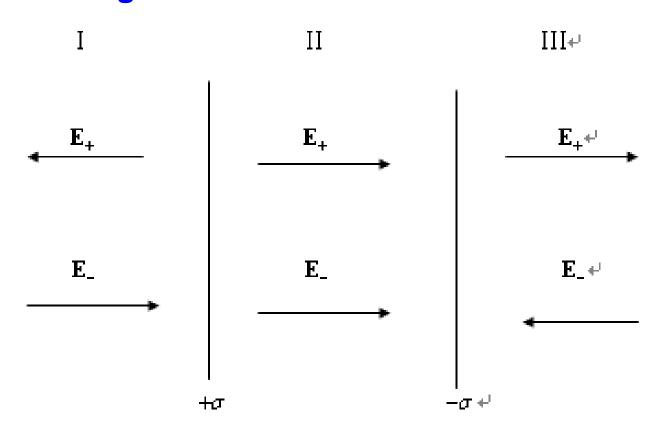
$E_{\downarrow}$ and  $E_{\perp}$  are the E fields due to the positively and negatively charged plane, respectively.
