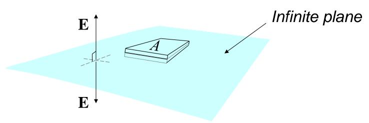
Without loss of generality, let the plane be the *x-y* plane. Then by symmetry, the E field above the plane is
