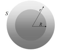
The situation is exactly the same as if the total charge, q, were located at the center.
