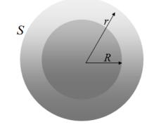
The situation is exactly the same as if the charge enclosed by S were located at the center and the charge outside S gave zero contribution.
