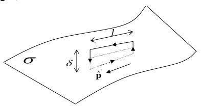
Consider the line integral of the **E field** along the rectangular loop. If we take  $\delta \rightarrow 0$  such that the contributions of the two short sides can be neglected.
