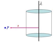
E field inside and outside an infinite long cylinder with radius R carrying a charge density  $\rho(s)$  which depends on s only.
