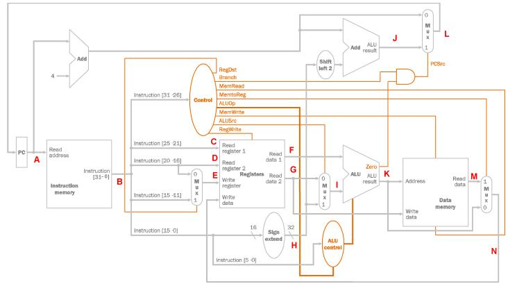
Question 1: Repeat the execution of the I-type instruction "SW \$t0, 8(\$t1)" by filling the values for A-N and also the control signals.
