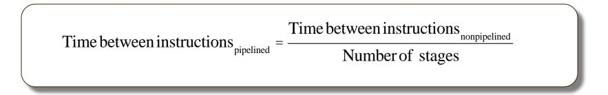
□ If the pipeline is well balanced, the **speedup** equals to Number of pipeline stages (a.k.a depth of the pipeline).
