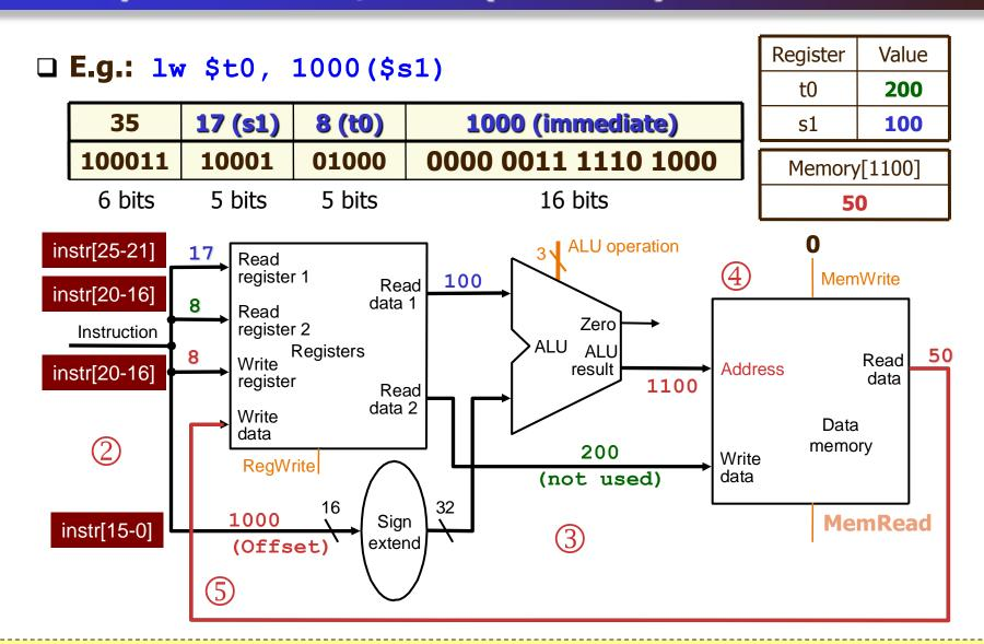
Note: For load word instruction, **MemWrite** has to be de-asserted so that the memory will not be modified by incoming write data.
