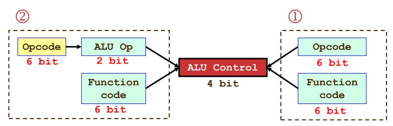
2 levels of decoding: only 8 inputs are used to generate 3 outputs in 2<sup>nd</sup> level
